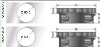
Position of the holes on the circular cable entries with diameters 50 and 63 mm
